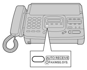
The FAX/MSG.SYS. indicator is on.
